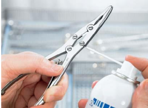
Oiling screws on an articulated instrument
