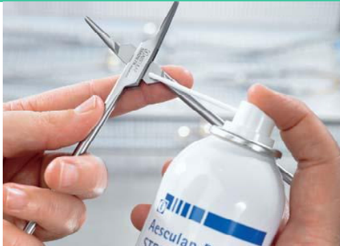
Oiling a box joint
